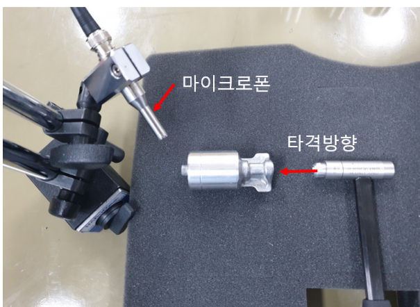
Fig. 8. Photograph of the setup to test the welding quality of the welded part. A manually operated hammer was used with a microphone located near the test sample.
