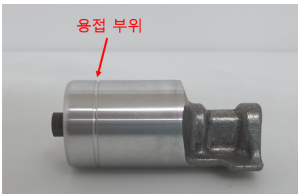
Fig. 7. The image of the test sample. The smooth welding line is shown. There was no visual appearance difference between the good welded and the ill welded parts.
