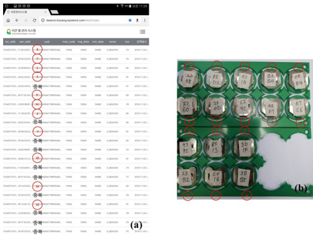
Fig. 7. Signal reception stability test of the beacon receiver. (a) A web page of location management platform; (b) Beacon signal transmitter.
