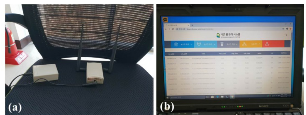
Fig. 6. Beacon signal transmission distance improvement test. (a) A reference receiver & Receiver with additional antenna; (b) A web page of location management platform.
