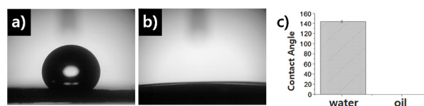
Fig. 5. (a) Water droplet on the membrane; (b) oil droplet on the membrane; (c) water/oil contact angle of PTFE membrane.
