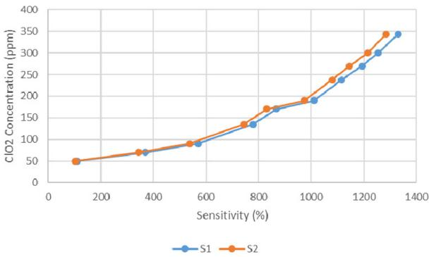
Fig. 7. Linearity for chlorine dioxide gas
