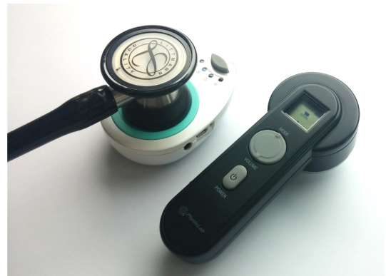
Fig. 1. Photograph of electronic stethoscope, Sound Share model from PhysioLab. Right part is transmitter and left part is receiver.
