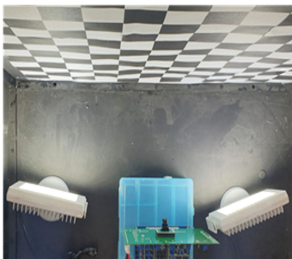
Fig. 8. Measurement system for image acquisition using proposed CMOS binary image sensor.
