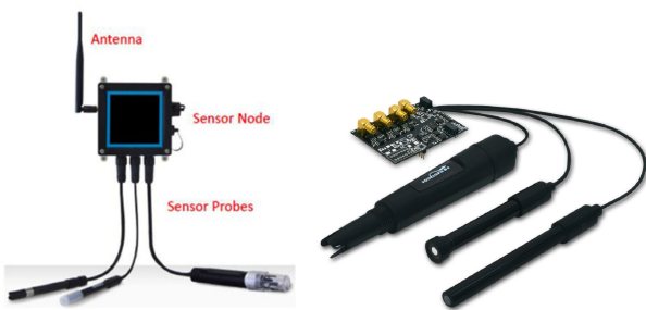
Fig. 5. IoT water quality sensor example [4].
