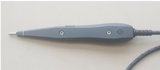
Fig. 13. Assembled pin type current probe.
