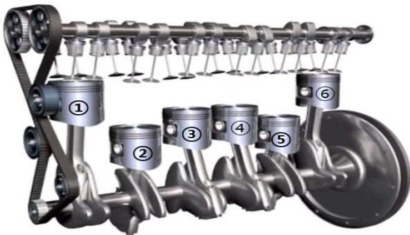
Fig. 1. Structure of In-line 6 piston engine.
