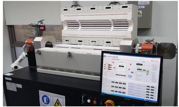
Fig. 4. Picture of thermal furnace used in SnO 2 thermal treatment process.
