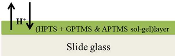
Fig. 4. Sensing layer cross-section HPTS.
