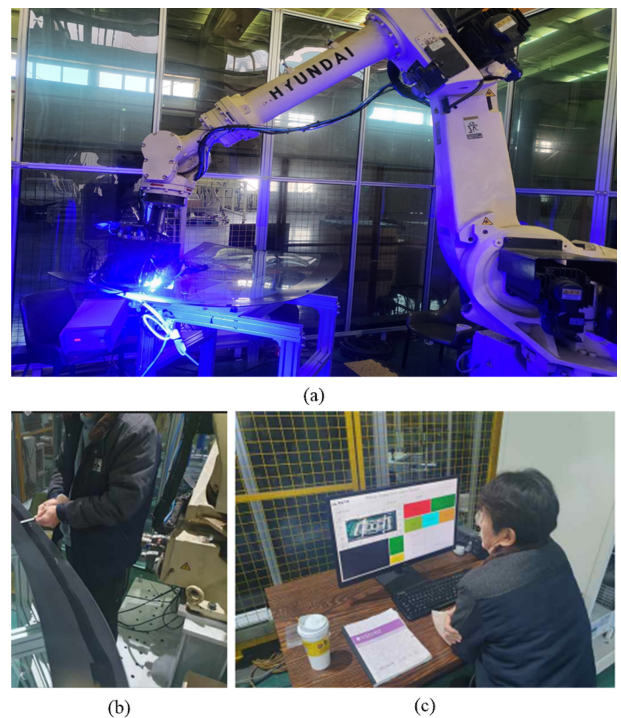
Fig. 10. Experimental environment for performance verification; (a) A real primer inspection test scene, (b) scene of measuring the width of the coating primer, and (c) a vision software of primer inspection test scene.
