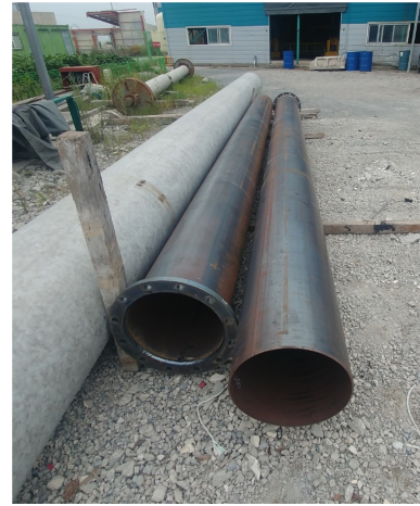
Fig. 10. Steel pipe specimen for testing
