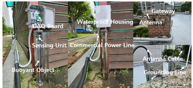
Fig. 10. An example of the testbed set up using a buoyancy-based level sensor and gateway.
