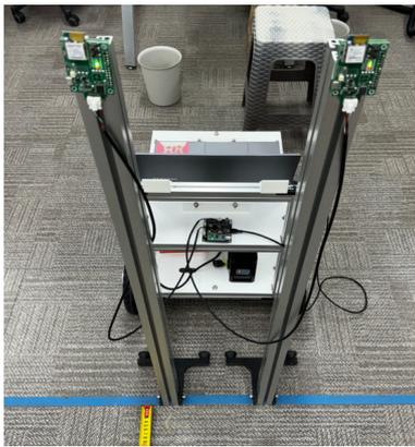
Fig. 5. Two fixed tags (left and right)
