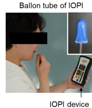
Fig. 3. IOPI device used to measure tongue pressure
